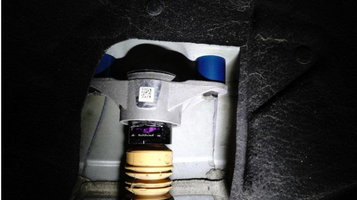
Rear damper installed in car with provided spacers and bolts.
