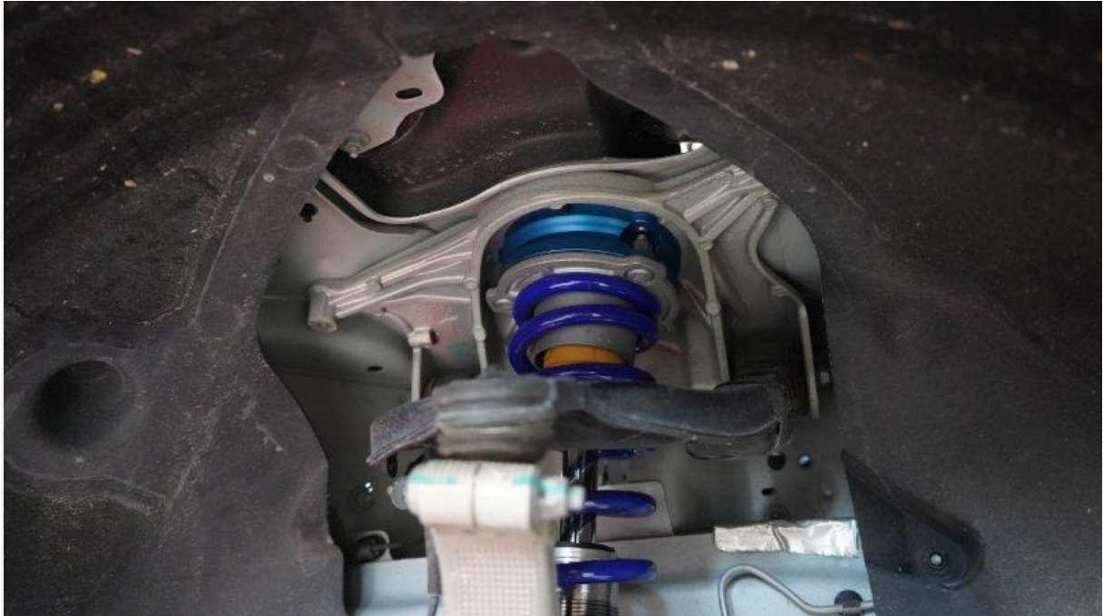
Front damper installed with lift kit spacer. Pretty isn't it?
