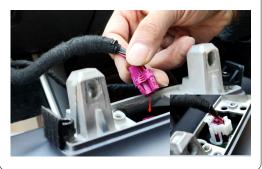
After recover, screen should be align with the bracket part shown in the arrow, find out the screw holes
