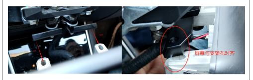
16 Use our screws with putting the mat, tighten the screws, and then use a 13mm Screw socket to further fix the screen and the bracket
