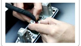
6 Lightly press the small buckles on both sides of the screen plug and unplug it (before operating this step, make sure the screen power is turned off)
