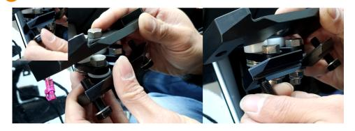
Parallel to insert the mount kit to the position of original car screen on the dashboard
